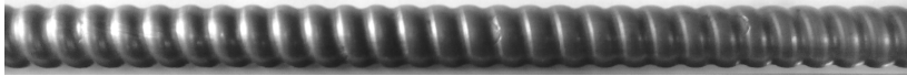
Fig. 1. Long dimensional screw-shaped tube (diameter 16 mm, step 8 mm), made in one pass
